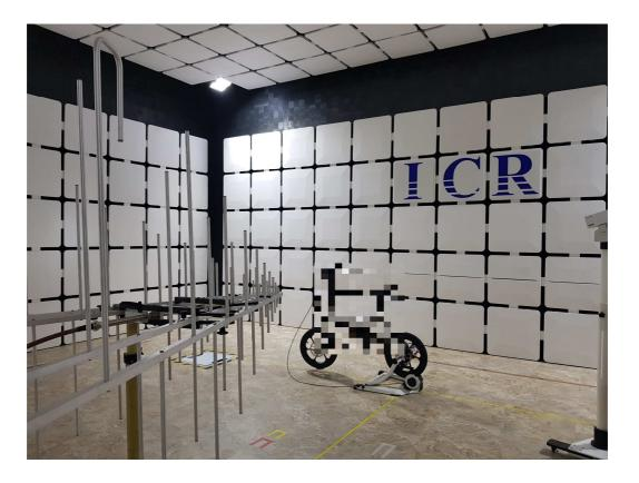
Our Power amplifier and Transmitter antennas support Radiated RF immunity testing for the KN 15194.
