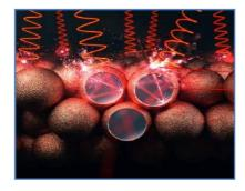
A state of the electromagnetic wave shielding material developed by the Korea Science and Technology Research Institute (Hokkaido University) The electric conductivity was enhanced by placing a hollow ball coated with copper in the polymer "polycaprolactone." provided by KIST
