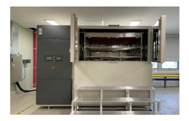
**■ ICR** has been operating two large Thermal shock tester.
