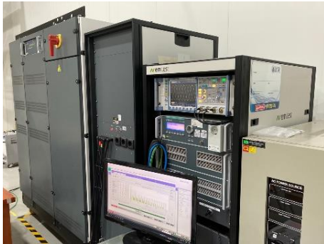
<Harmonic Current Emission Test Equipment> <Low Frequency Signal Immunity Test Equipment>
