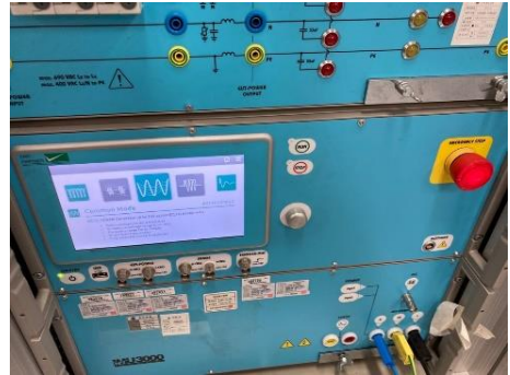
<Harmonic Current Emission Test Equipment> <Low Frequency Signal Immunity Test Equipment>
