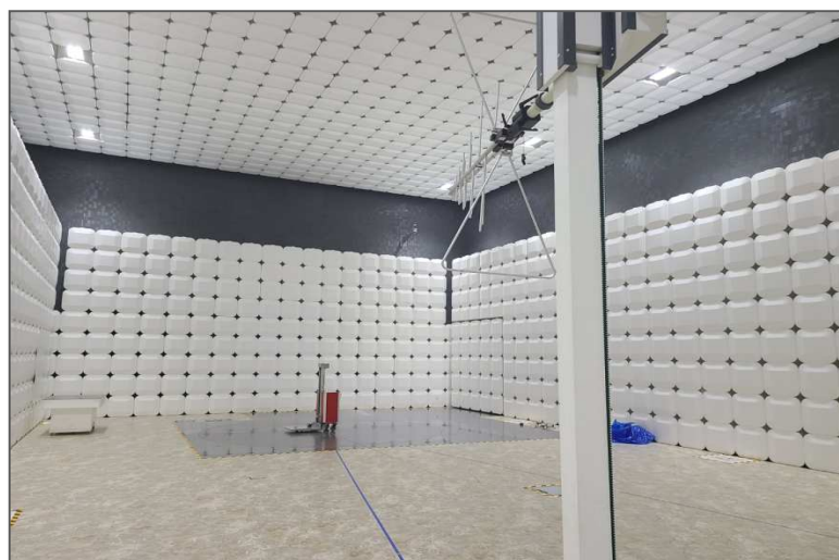
< Electromagnetic disturbances test >
