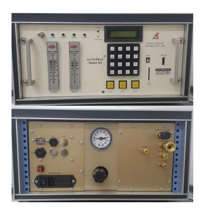
The ICR has a detection device (AUTOTRACK) for detecting trace gases and provides a test for the leakage of trace gases specified in SEMI S6 for chemical facilities using hazardous materials.
